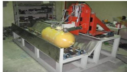
Fig. 3. The mechanism of type 'b' for ultrasonic testing system
