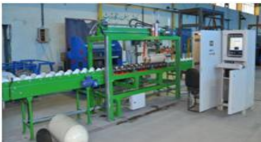
Fig. 4. The mechanism of type 'c' for ultrasonic testing system
